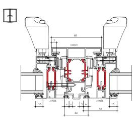
U-Value (Double Glazing) - Windows are calculated using EN ISO 10077 - Part 2, 1230mm x 1480mm Side hung next to fixed light with Ug: 1.0 W/m²K using AW603 outerframe and AW614 ventU-Value (Triple Glazing) - Windows are calculated using EN ISO 10077 - Part 2, 1230mm x 1480mm Side hung next to fixed light with Ug: 0.7 W/m²K using AW603 outerframe and AW685
