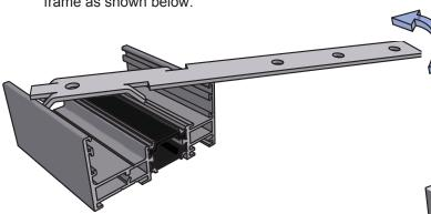
Take the fixing lug (XA947) and position against the outer edge of the frame to be fixed.
