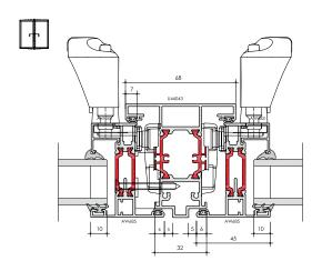
U-Value (Double Glazing) - Windows are calculated using EN ISO 10077 - Part 2, 1230mm x 1480mm Side hung next to fixed light with Ug: 1.0 W/m²K using AW603 outerframe and AW614 ventU-Value (Triple Glazing) - Windows are calculated using EN ISO 10077 - Part 2, 1230mm x 1480mm Side hung next to fixed light with Ug: 0.7 W/m²K using AW603 outerframe and AW685 vent
